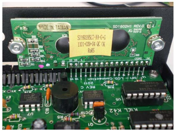
10) Now sneak in with a soldering iron and solder two pins at each end of the connector. I recommend soldering the fourth pin in from each end.
