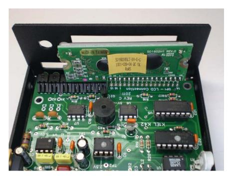
9) Use two 4-40 nuts with lockwashers (from the original assembly) to hold the display in place. Before tightening the nuts make sure the display is centered in the enclosure window. Line up top and bottom, left and right, and check that the display is not crooked. When you are sure this is correct, tighten the display holding nuts. It can be helpful to center the mounting stud in the display cutout ahead of time.
