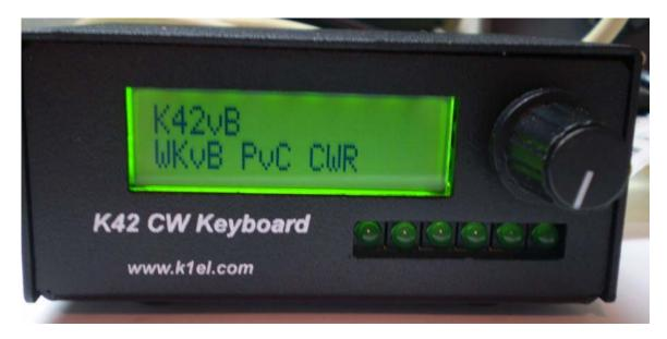
This document describes how to upgrade the K42 Rev A CW Keyboard kit. There are two parts of the kit that will be upgraded; the first is the LCD display will be swapped out to one that has backlight. The second will be upgrading the PsoC controller to one that provides much better CW reader performance.
