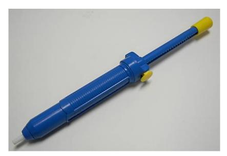
It is also possible to do this with Solder-Wick or a vacuum desoldering tool.
