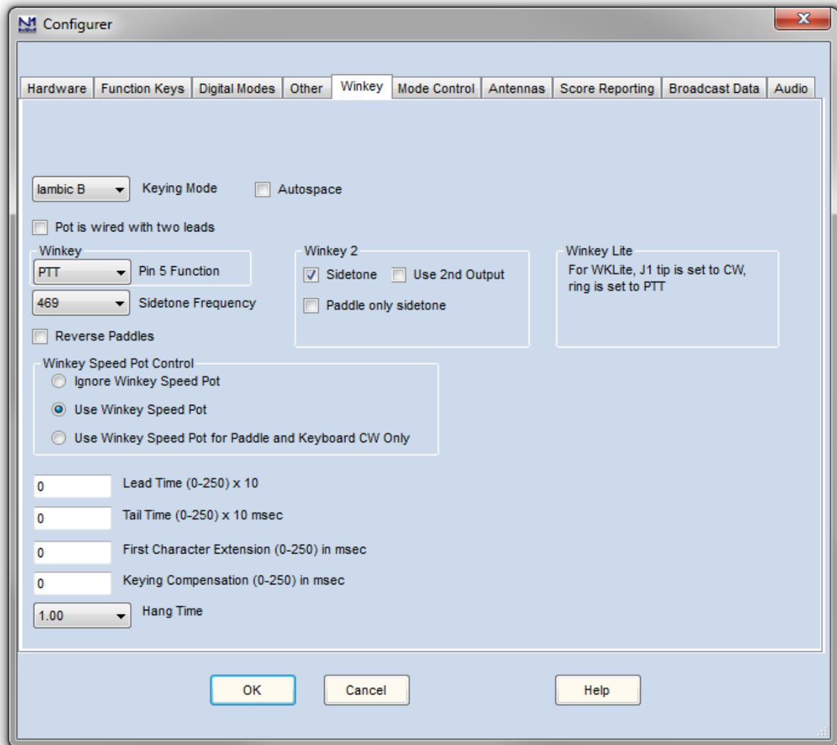
There are very descriptive hints on most of the controls. The Winkey 2 options also apply to WK3 based keys. Disable Paddle Only Sidetone for initial testing purposes.
