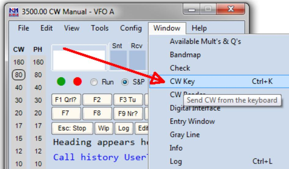
The CW keyboard window is now displayed and you can type into it to send letters to WKUSB. Note that when the Send CW window is up, the main N1MM+ dialog box is disabled. For a final test, turn the speed pot and you should see the CW Speed display in the main N1MM+ dialog box change. (This assumes that the speed pot has been enabled in the Winkey configuration dialog box)
