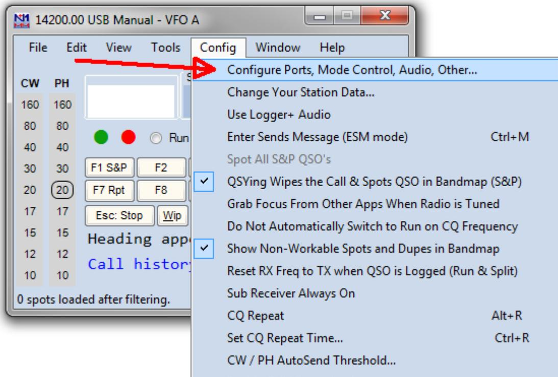
This brings up the port configuration dialog box. This is where all the different devices attached to N1MM+ are set up.
