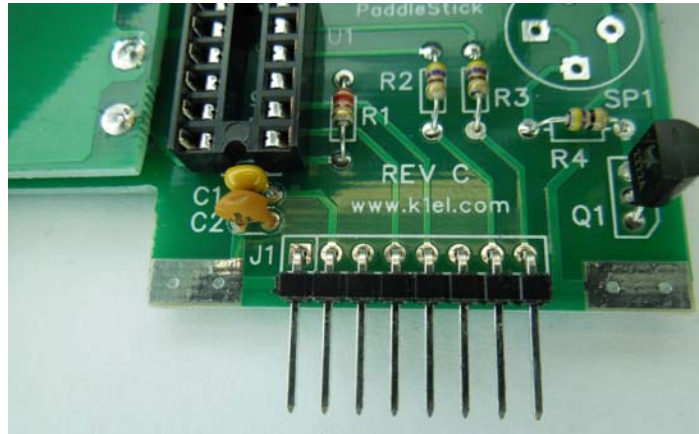
Figure 12 – 8 pin header in place
