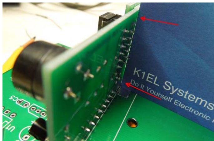
Figure 16 – Verify that the PS is at a right angle to the PSB
