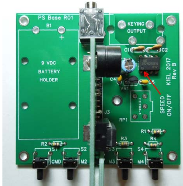
Figure 22 – PSbase components installed
