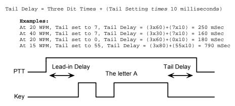
Figure 5 – PTT Lead-in and Tail Example
