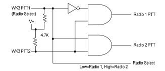
The PTT outputs on WKUSB are open collector so pull up resistors are required to generate logic high and low conditions. PTT1 will be logic zero when radio 1 is selected and logic one when radio 2 is selected.
