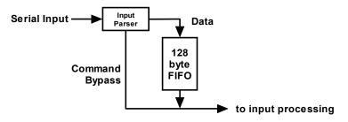
Figure 3 – Data and Command Flow inside WK3
