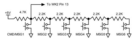
Figure 9 – Pushbutton Matrix
