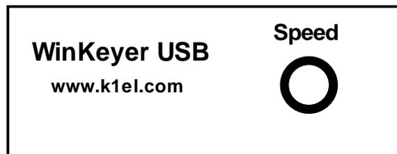
There is one knob that is used to set WKUSB's operational WPM rate. In standalone mode the knob will always control speed. In host mode the speed control may or may not have an affect depending on how the app is configured. Some applications only allow you to change the speed by their own controls and will ignore WKUSB's control.
