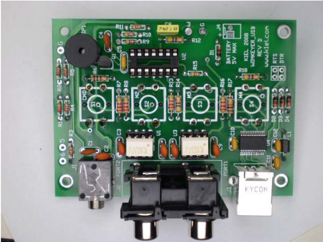
Completed WKUSB Rev D PCB
