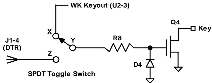
Figure 11 – Key Out Source Switching Option
