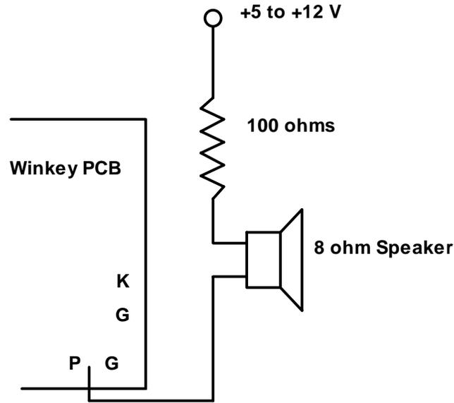
Figure 10 - Sidetone Connection for WinKey PCB
