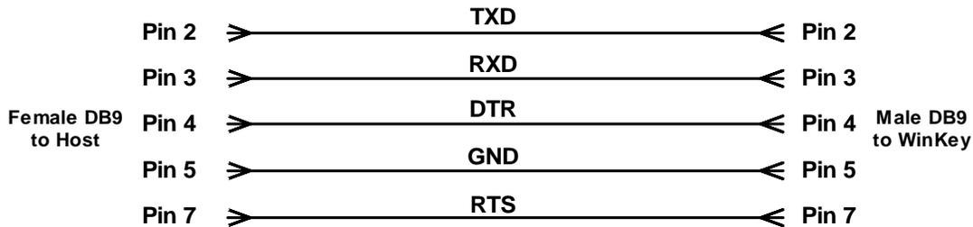
Figure 3 – WinKey RS232 Interface Cable Schematic
