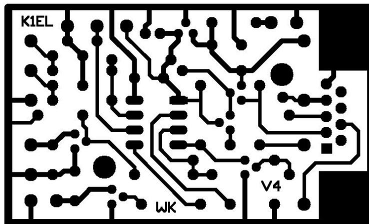
Figure 7 - WinKey PCB Solder Side
