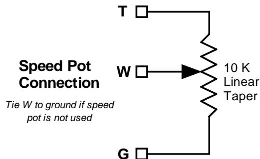
Figure 2 – Speed pot Connection
