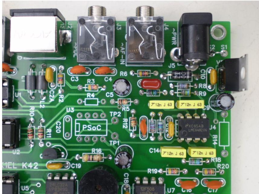
11) We can't test the AF filter until the PSoC processor is installed, we will do that now
