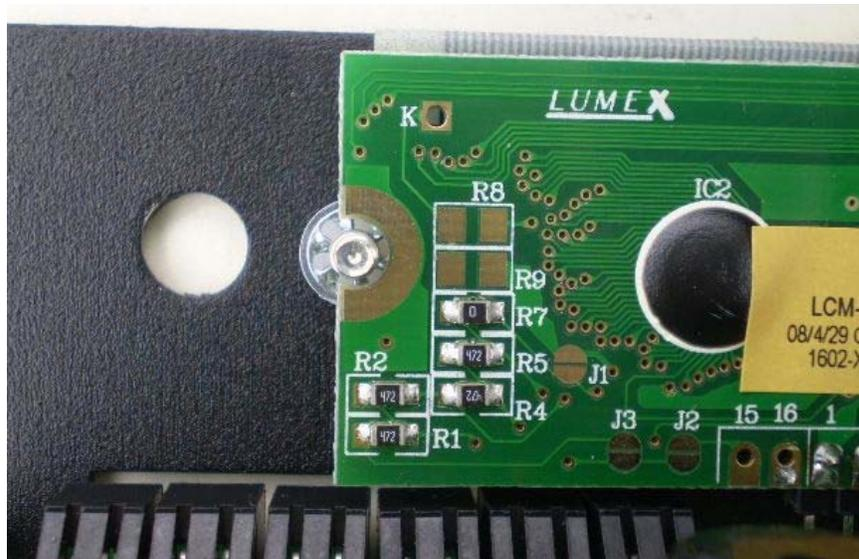
Adjust the display so the threaded studs are centered in the display's mounting holes as shown. Then place a star washer one each side followed by 4-40 nuts then tighten just enough to hold the display in place.
