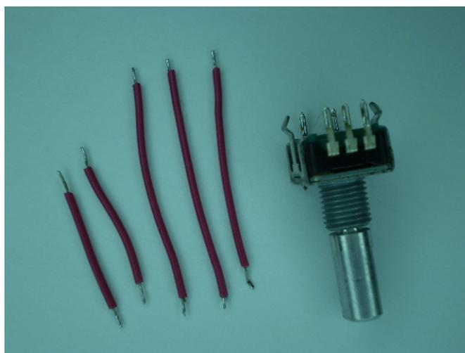
Prepare five wires, two are 1 inch long the remaining three are 2 inches long. Strip and tin both ends as shown in the picture.
