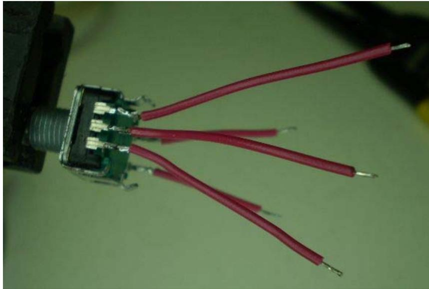
Next tin the five leads on the encoder and attach the five wires, short ones to the side with two lugs (X1 and X2) and the three long wires to the side with three lugs. ( E1, E2, and E3).
