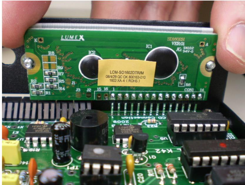
Then fold the display up into place on the threaded studs
