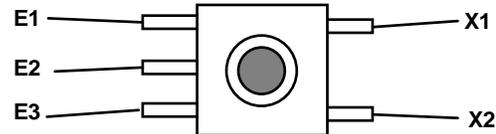
The drawing above shows how the wires should be connected to pads on the K42 PCB board. E1, E2 and E3 are the encoder outputs while X1 and X2 are the encoder's pushbutton switch connections
