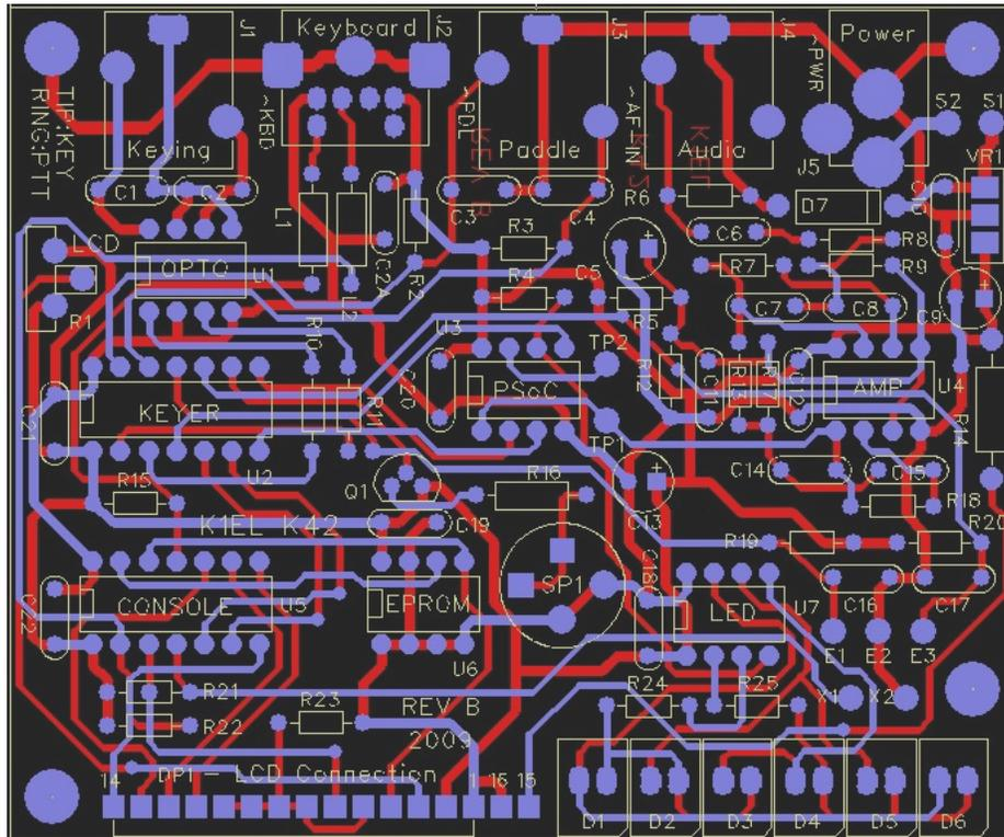
Figure 4 - K42 Composite Checkplot, Red=Bottom, Blue=Top
