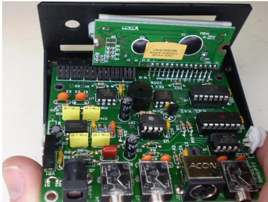
Now carefully remove the LCD display/K42 PCB assembly and solder the remaining header pins from the bottom of the K42 board. **SOLDER THE TACKED JOINTS LAST** to preserve your alignment.
