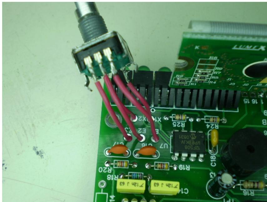
Then solder the remaining three wires: E1, E2, and E3
