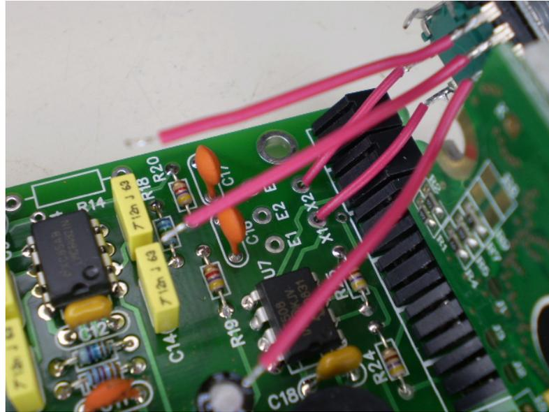
Solder in the X1 and X2 wires first
