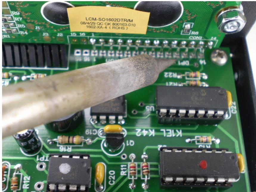
Make sure the K42 PC board is firmly seated on the enclosure standoffs and that the display is held firmly in place by the 4-40 nuts. Now very carefully sneak in with your soldering iron and tack solder two pins on the header to the K42 main board as shown. Solder the fourth pin in from each end, being careful that the barrel of your soldering iron does not come in contact with anything.
