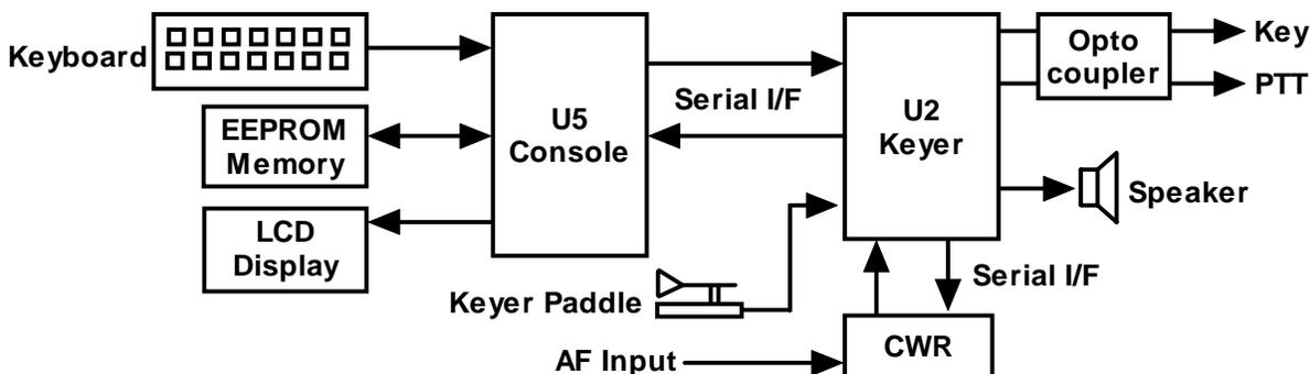
Figure 1 - K42 CW Keyboard Block Diagram
