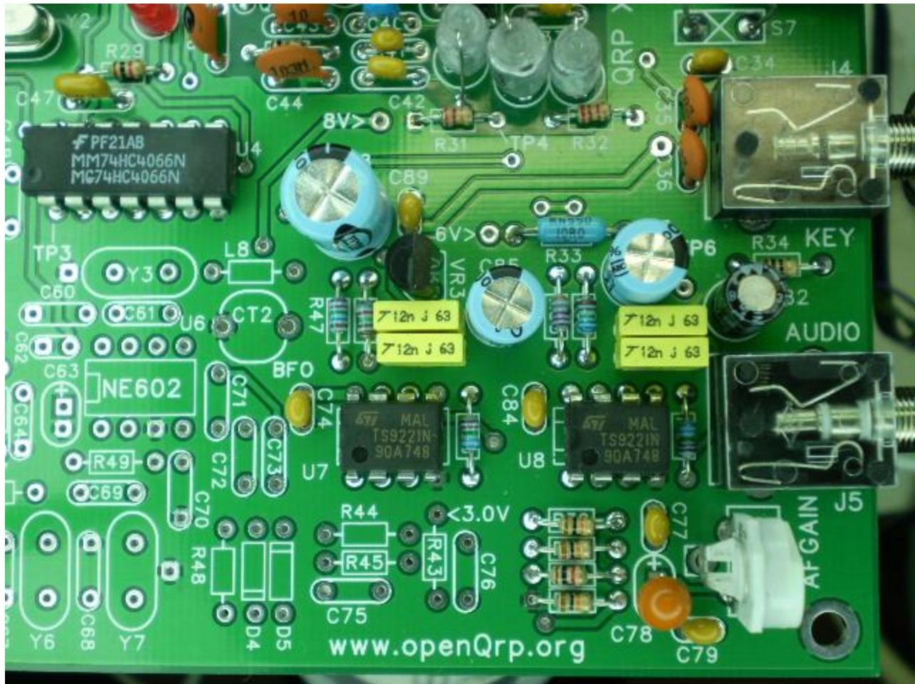
Audio amplifier and active filter installed, the analog switch can be seen in upper left.
